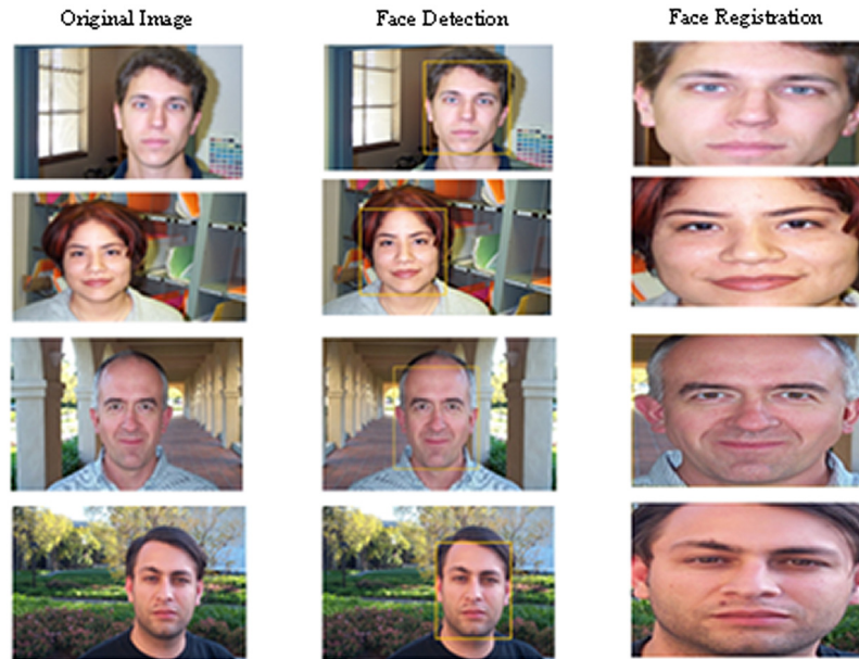
Fig. 3. Face detection and cropping using the Viola Jones algorithm.
