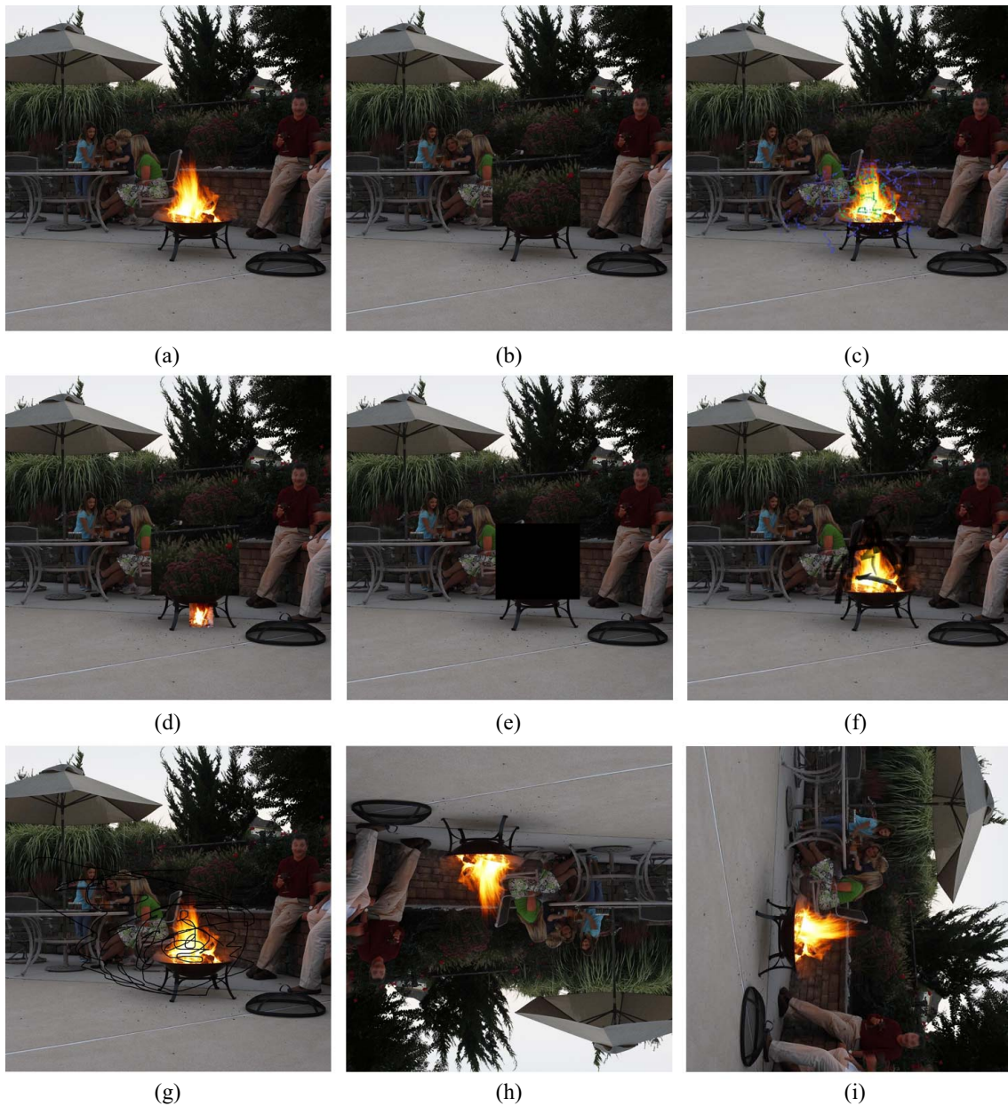
Fig. 11. Evaluation of the robustness of the proposed fire detection algorithm against different attacks (noise, cropping, and rotation); images (b) and (e) are labeled as normal, and the remaining seven images are labeled as fire. (a) Test image (Fire: 99.24%, Normal: 0.76%). (b) Normal: 99.9%, Fire: 0.1%. (c) Normal: 5.99%, Fire: 94.01%. (d) Normal: 21.89%, Fire: 78.11%. (e) Normal: 99.88%, Fire: 0.12%. (f) Normal: 15.15%, Fire: 84.85%. (g) Normal: 9.94%, Fire: 90.06%. (h) Normal: 28.89%, Fire: 71.11%. (i) Normal: 0.37%, Fire: 99.63%.
